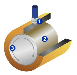
Proper lubrication will prevent the need for replacement or repair of pin bushings, except in case of bushing deformation due to impact loading. Manual lubrication typically produces inconsistent lubrication. This allows contaminants to enter the bearing, producing premature wear and impacting bearing life significantly.
